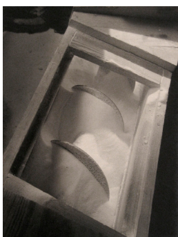
3 Harold Haliday Costain The Archimedean Screw Carries the Evaporated Salt from the Dryer to the Storage Bins, Avery Island, Louisiana 1934 Chlorobromide Print 14" x 10.75"
