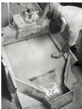
4 Harold Haliday Costain Electric Vibrating Screen Used in Grading the Salt, Avery Island, Louisiana 1934 Chlorobromide Print 13.75" x 10.75"
