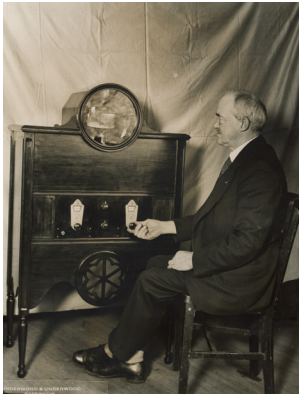
5 Underwood & Underwood In June 13, 1925, inventor Dr. C. Francis Jenkins publicly demonstrated synchronized transmission of pictures and sound Washington D.C. 1929 Gelatin Silver Print 10" x 7.5"
